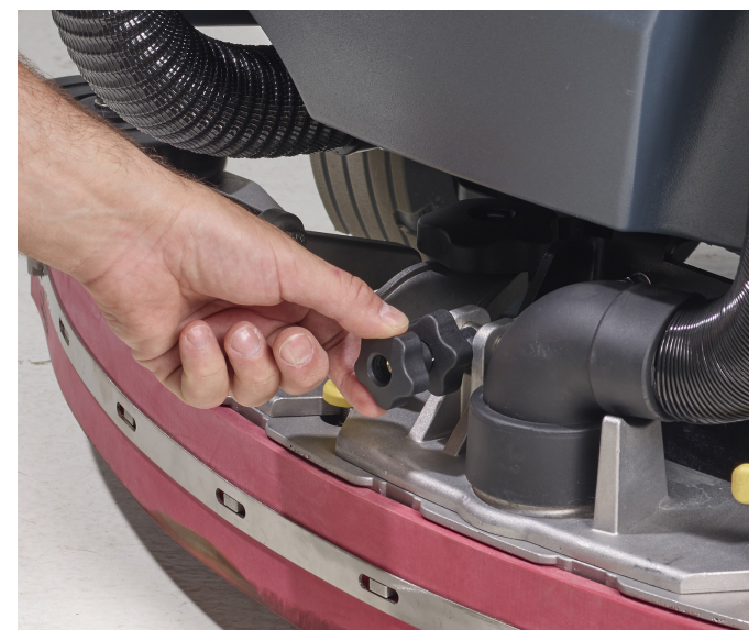
7. Check the height of the squeegee by adjusting the castor wheels and the angle knob.
