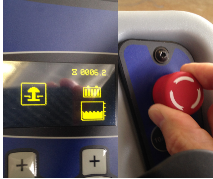
2. E-stop icon that appears on display when E-stop switch is engaged. Twist E-stop switch to enable machine function
