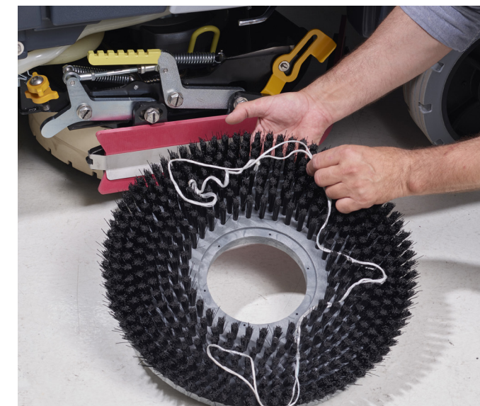
8. Open broom door compartment and check presence of ropes or debris that can block it.
