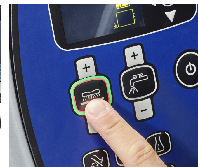
14. Make sure that deck and squeegee are moving down when pressing the button.
